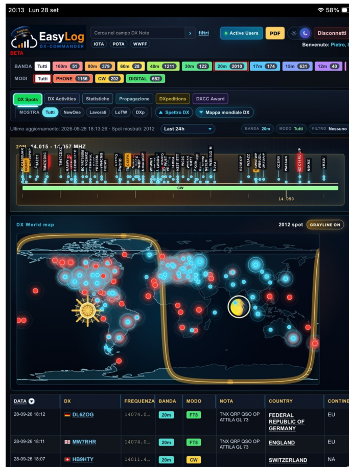
Figure 4 DX spectrum of the selected band and world map with Grayline
